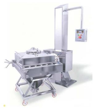
Ideal equipment for blending within a closed environment and dust free operation. The Quality of the blending is achieved by the shape of the container without any internal baffles. The unit is most suitable for handling of different size containers by using a common drive.
